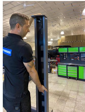
8. Attach the post cap check that the hole for the wire matches how the wire wheels are positioned. There should also be a nut with a washer on the crampom that should be on the underside of the cap.
