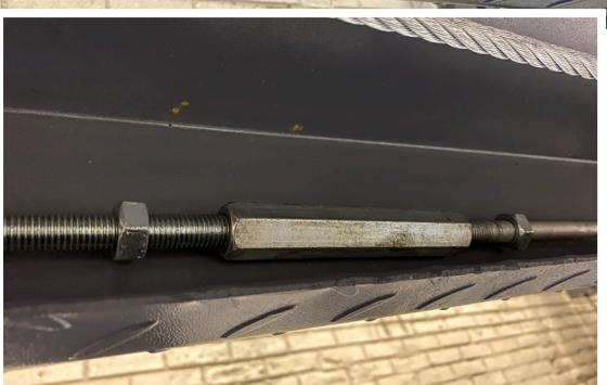
27. Mount the shaft to the latches remember to place the handle where the pump unit is located. Insert the other shaft from the other side and assemble them on the underside of the ramp.
