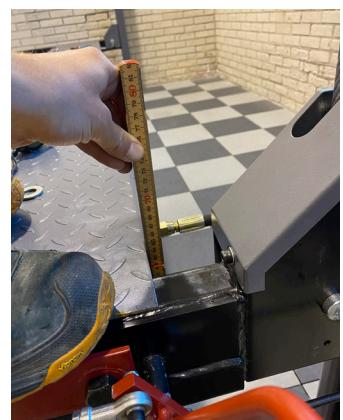
31. Fit the loop screw for the long linkage and thread it through.
