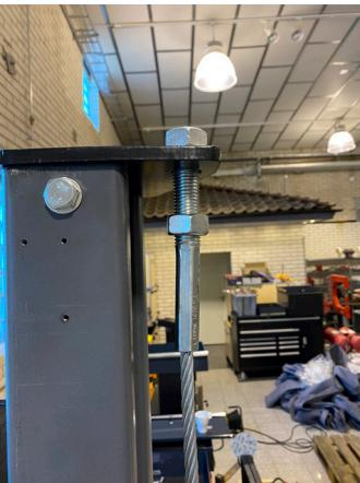
32. Stretch the wires so that the catches click at the same time when you raise the ramps.
