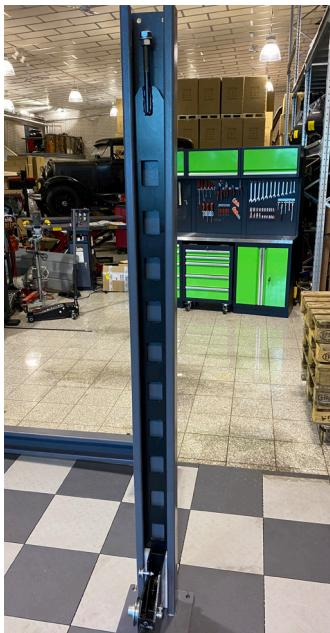
6. Install the crampoms in which the catches are to be locked.
