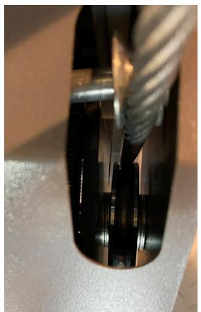
19. Thread the wire through the cover. Thread the wires so that they are as shown in the picture above. The small wire wheel causes the latch to enter the latch-ladder if a wire comes off.
